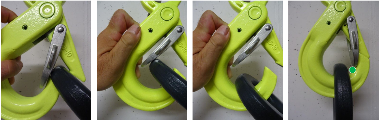
Fig. 18 – 21: Open the hook and insert the fitting or thimble. Leave the hook open and fully insert the black fitting. The fitting is correctly placed only when the 2nd safety latch is completely closed.
