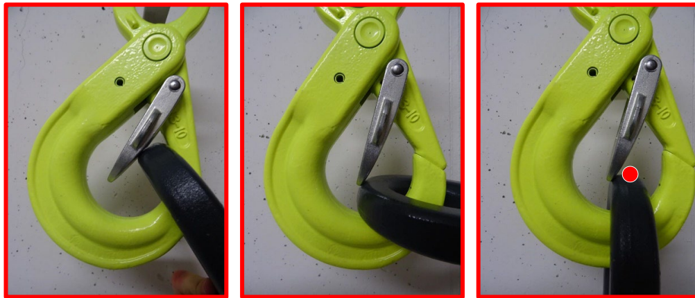
Fig: 22 – 24: Misuse! If the hook aperture is closed immediately after having inserted the black fitting, the safety latch cannot be appropriately locked.
