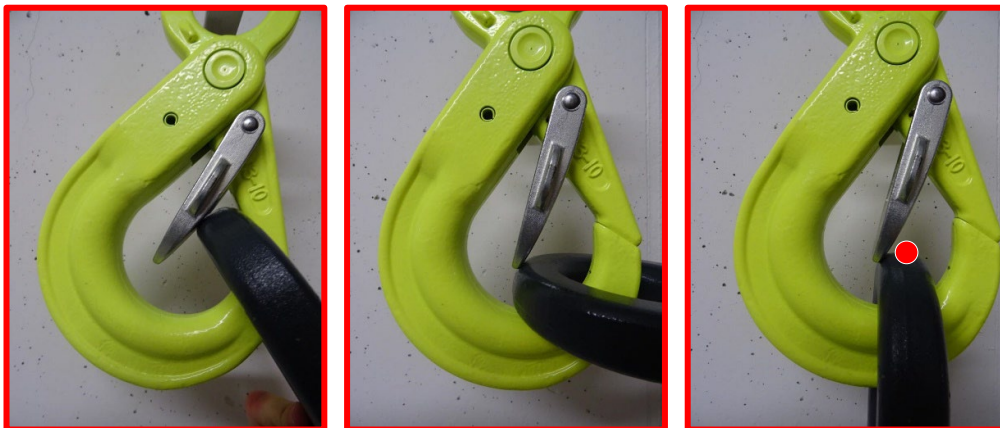
Fig: 15 – 17: Misuse! If the hook aperture is closed immediately after having inserted the black fitting, the safety latch cannot be appropriately locked.
