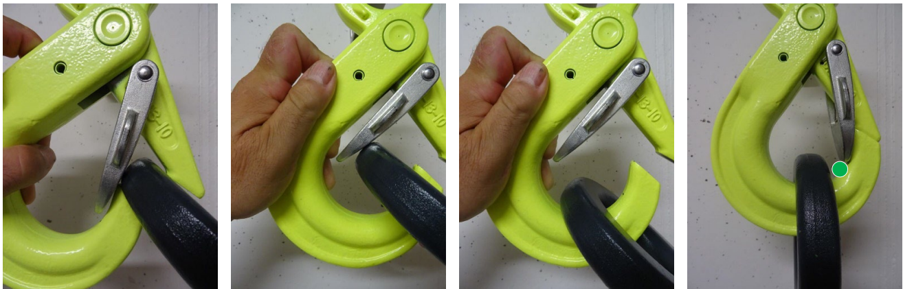
Fig. 11 – 14: Open the hook and insert the fitting or thimble. Leave the hook open and fully insert the black fitting. The fitting is correctly placed only when the 2nd safety catch is completely closed.
